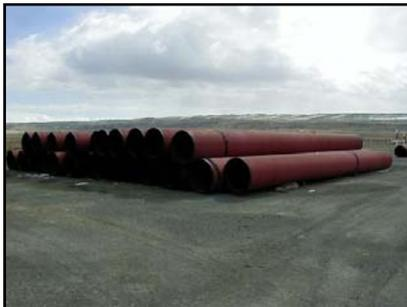
Line Pipe, 20in to 36in, 0.282in WT to 0.60in WT, 71.5# to 2227.06#, FBE, Bare or Tape Wrapped, 64jts, Unused
