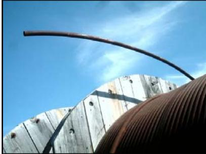
(Approx 7066ft) 1-1/4in Coiled Tubing, 0.110in Outer Wrap WT, 0.148in Bed Wrap WT, (Wall thicknesses are backwards on reel), 112in Spool Size, CGU 22-14, QTI# 27792, STR# Q27792
